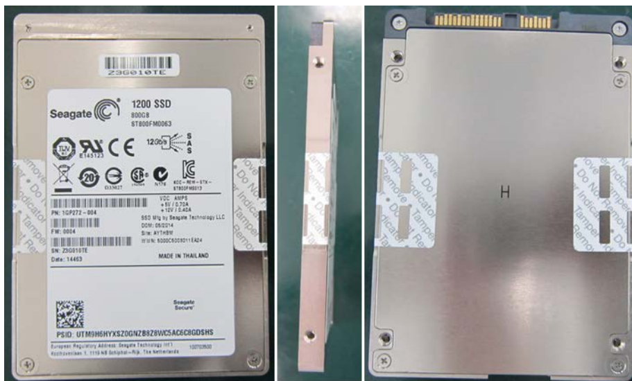
Figure 7 Example of FIPS tamper evidence labels
