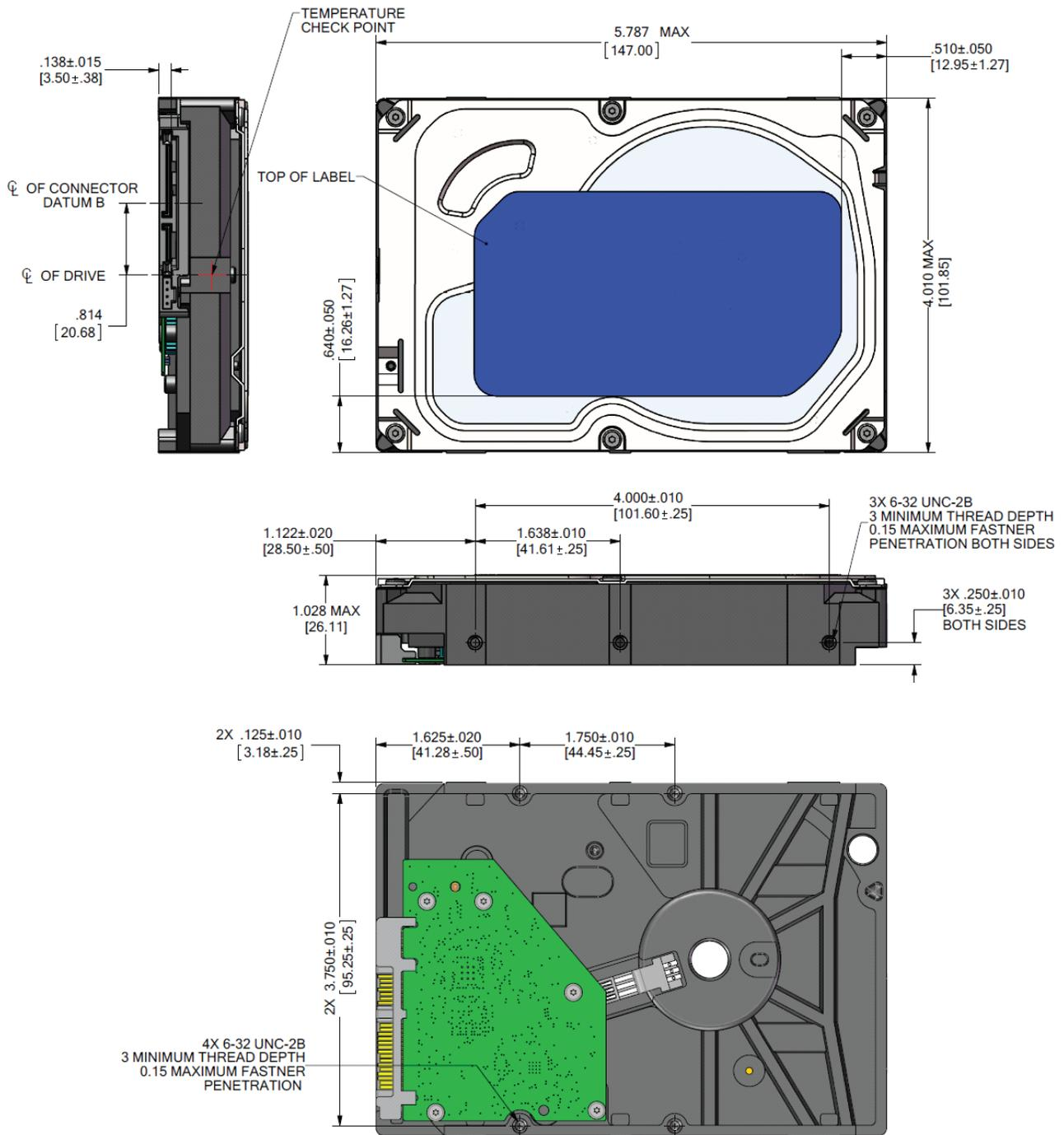
Figure 7 Mounting dimensions (3TB - 2TB)
