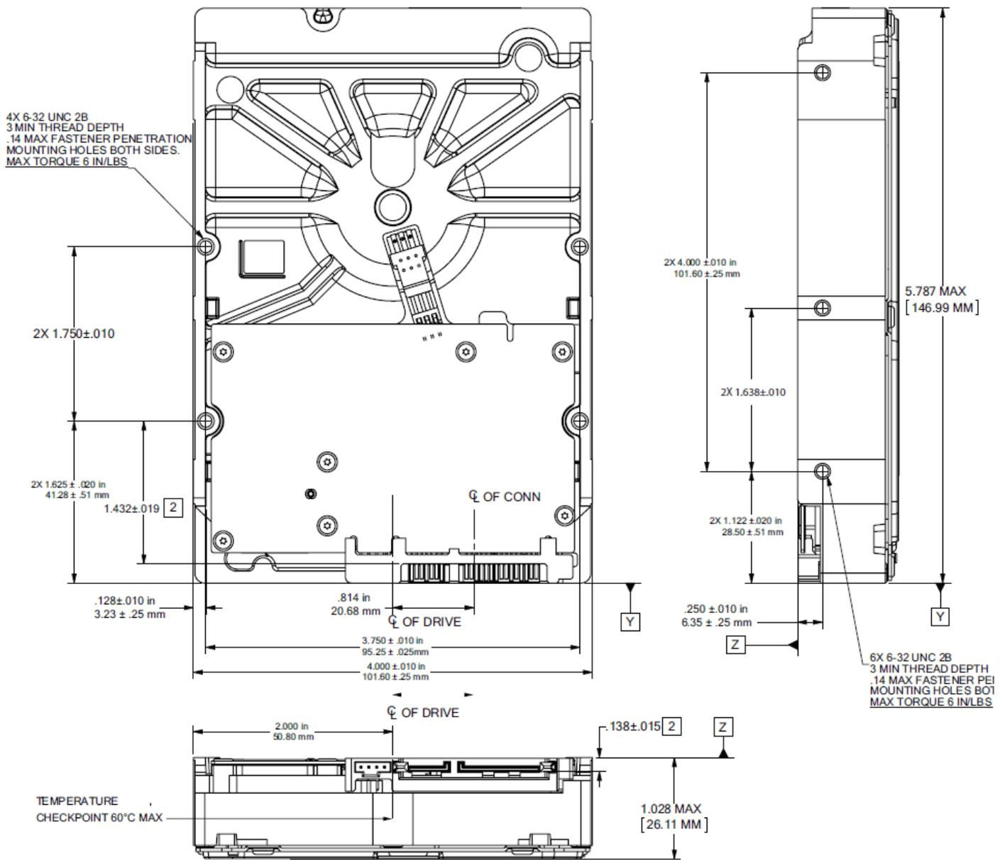
Figure 6 Mounting dimensions (4TB)
