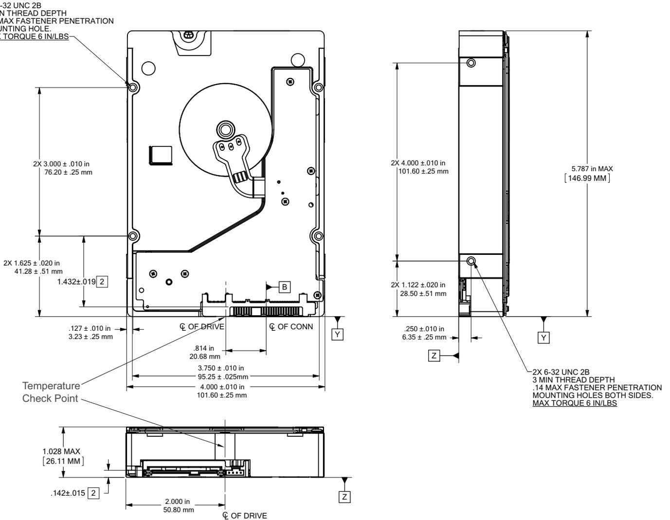
Figure 5 Mounting dimensions (6TB)
