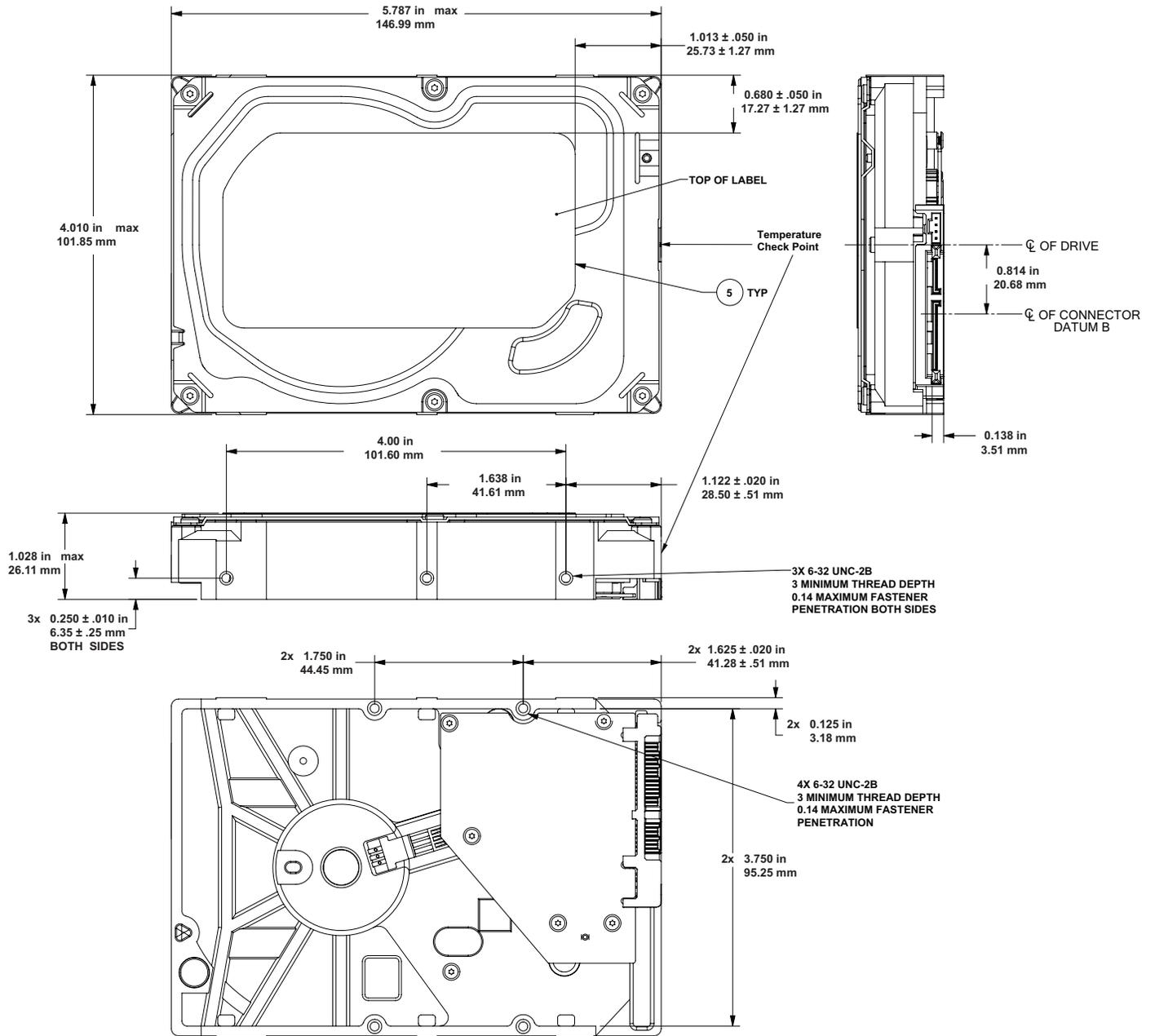
Figure 8 Mounting dimensions (1TB)
