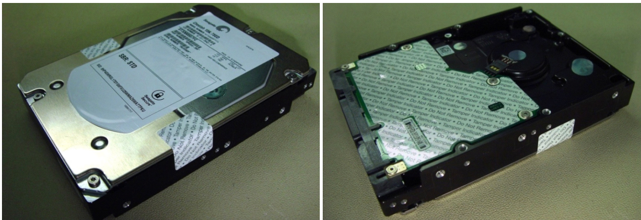
Figure 12. Example of FIPS tamper evidence labels/seals.
