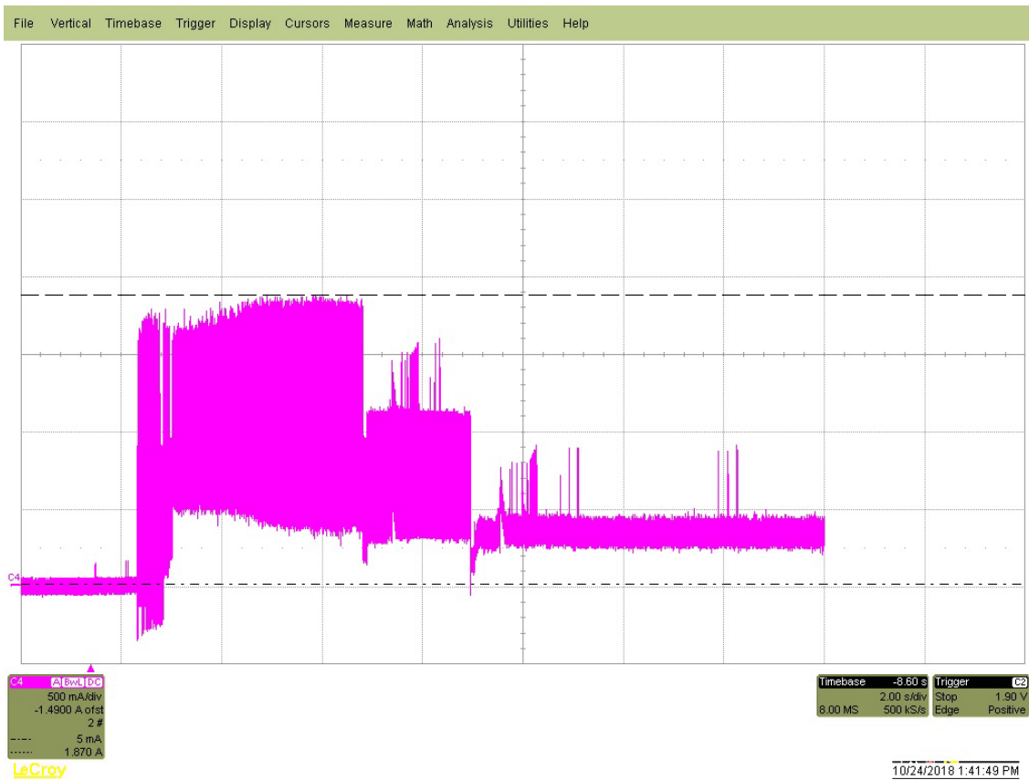
Figure 3. 2TB Typical 12V startup and operation current profile
