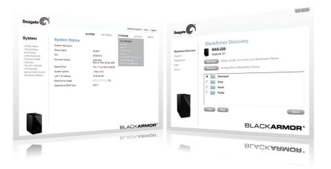
The BlackArmor® NAS 220 storage server can also function as an FTP server, allowing remote access to files. Using the web-based management interface, you can designate user access manually or integrate with Microsoft® Active Directory to populate users and groups...
